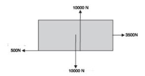
Figure 1: Force diagram of forces on caravan
