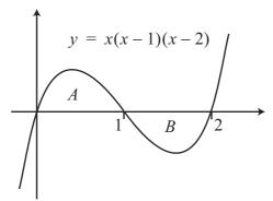
Now the areas required are obviously the area A between x = 0 and x = 1, and the area B between x = 1 and x = 2. But there is a marked difference between these two areas in terms of their position. The area A is above the x-axis, whereas the area B is below it. In previous units we have talked only about calculating areas using integration when the curve, and thus the area, is above the x-axis. Does the position of the curve make any difference to the area?
