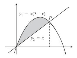
We can see that the distance between the two curves at any value of x is  $y_1 - y_2$ . Thus a small piece of the area between the two curves and the ordinates x and  $x + \delta x$  is  $(y_1 - y_2)\delta x$ . So we can add these small pieces of area together to get
